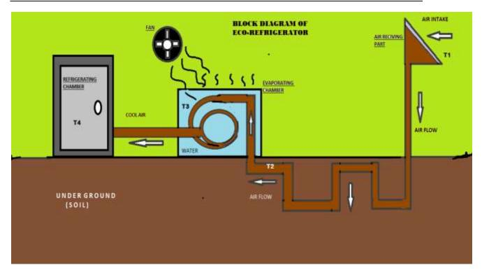
Fig1:- Block diagram of Eco-Refrigerator
